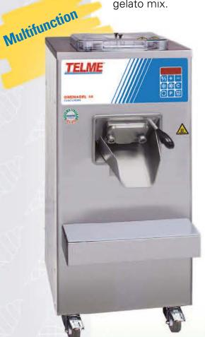
The temperature settings are adjustable and the thermal treatments are performed in a single cylinder to ensure best hygiene. The cylinder is vertical which means it is easy to fill, the product is always visible and ingredients can be added at any time.
